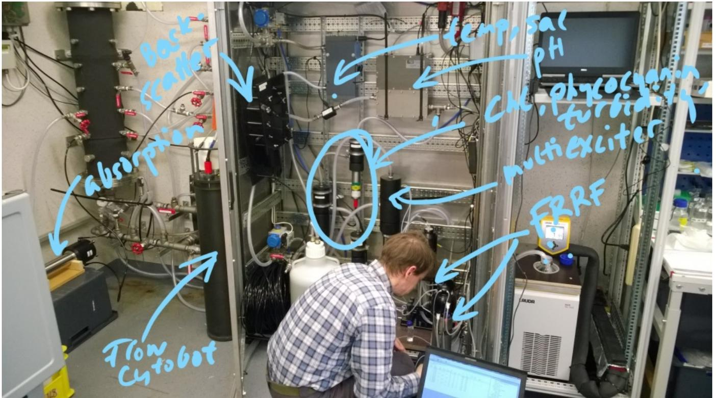
Fig. 3. And in reality, it looks like this (part of the automated Utö Marine Research Station). The AquaBox will require considerable downscaling, but the control and data acquisition software are scale-independent, so synergy with previous systems is essential for the AquaBox R&D work.
