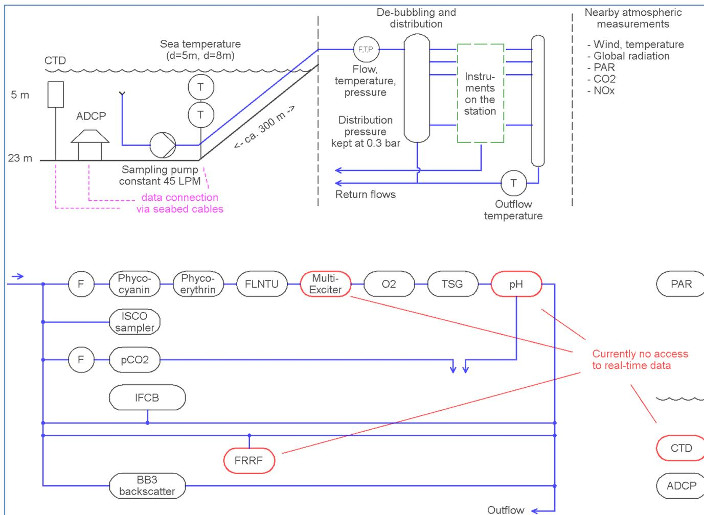
Fig. 2. Scheme of the automated Utö Marine Research Station. Control and data acquisition software are scripted in Python. All data are remotely accessible in real time except for notifications in red.
